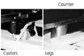
**Counters fitted with castors** – Remove fittings from inside the unit and ensure all drawers and doors are locked before removal from the pallet. Cut the heavy duty cable ties that hold the front castors to the pallet. Unlock the castors and then carefully roll the unit forward off the pallet.
