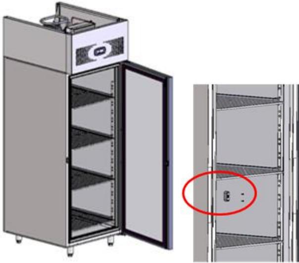
2. Remove the self-tapping screw that retains the unit cover and top surround using a screw driver.
