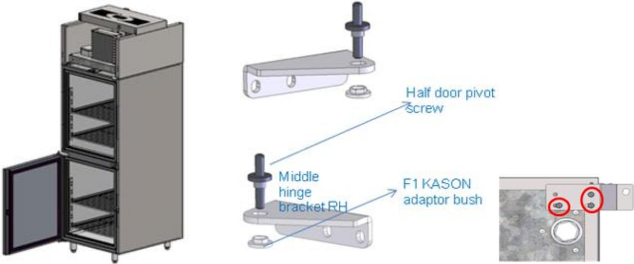
7. Fit the bottom door and top hinge bracket
