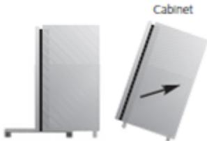
**Cabinet removal from the pallet:** Remove the shelf holding the package containing the castors. Remove the retaining bolts, which secure the unit to the pallet. Move the unit over the front of the pallet to fit the lockable castors in the mounting holes. To fit the rear castors, lock the front castors, tilt the unit forwards, remove the pallet and fit the castors in the mounting holes. Ensure that all are tightened firmly into position. This requires 2 persons.
