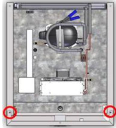
3. Remove the unit cover and lay on top of the unit. **DO NOT disconnect any wiring.**
